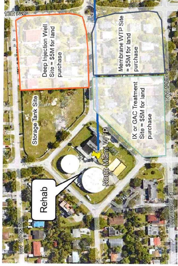
Rehab Lime Softening + Membrane Treatment at Winson Options
